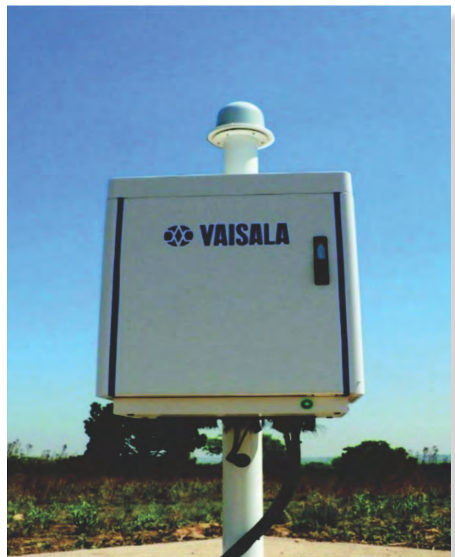
Lightning detectors form part of the SAWS Lightning Detection Network (LDN).
